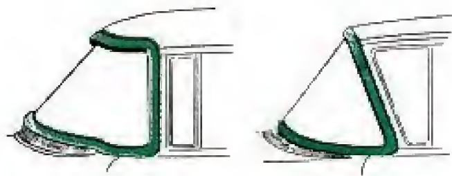
BUICK front corner pillars are vertical (left) on Super and Roadmaster, slanted on Special and Century
